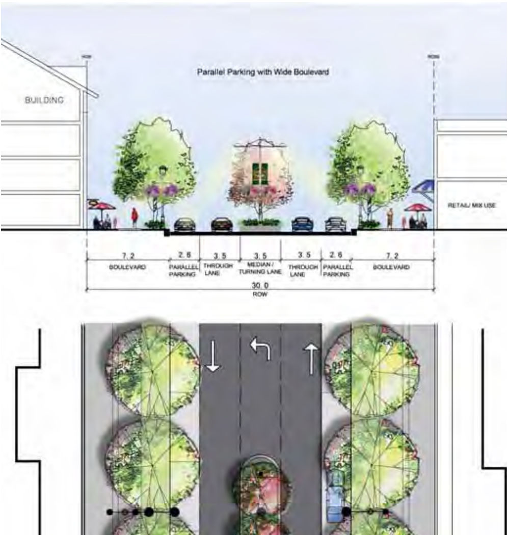
Figure 15: Parallel Parking with Wide Pedestrian Boulevard
