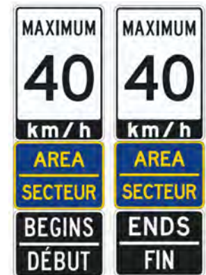
Figure 4-5 | Reduced Speed Gateway Signage
