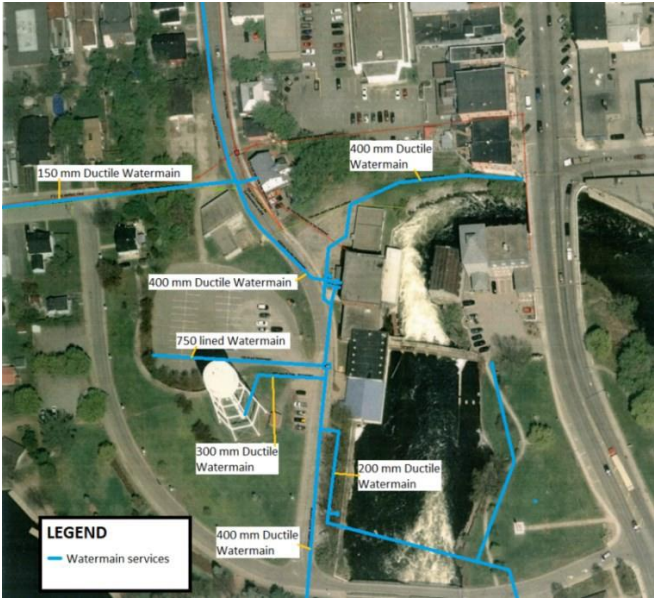
Figure 7: Water main Services
